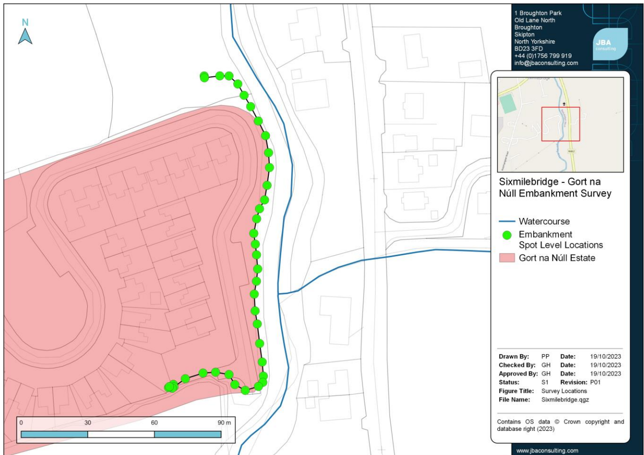
Figure 4-4: Additional survey- Gort na Núll Embankment
